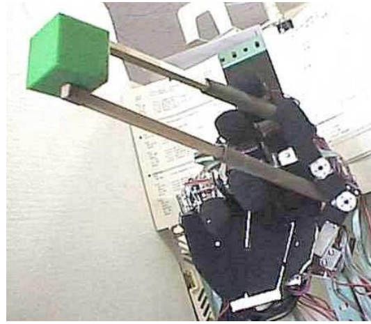
Fig. 19. The photo. of right hand in picking a sponge cube by chopsticks.
