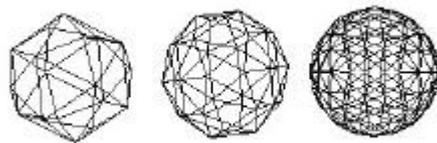
**Fig. 6.** Representing a sphere with 32, 48, and 192 polygons.
