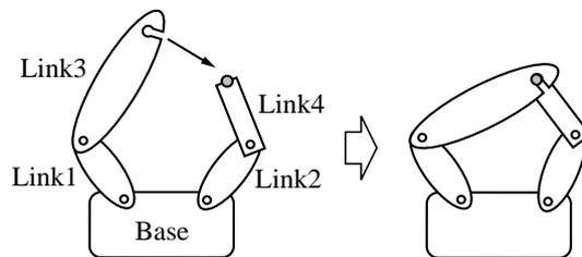
Fig. 4. Example of link connection
