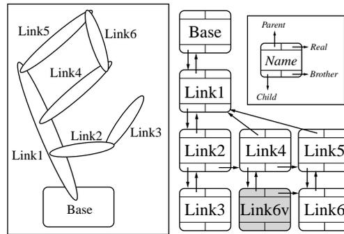
Fig. 3. Example of describing link structure
