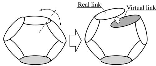
Fig. 2. Describing closed loop by virtual link
