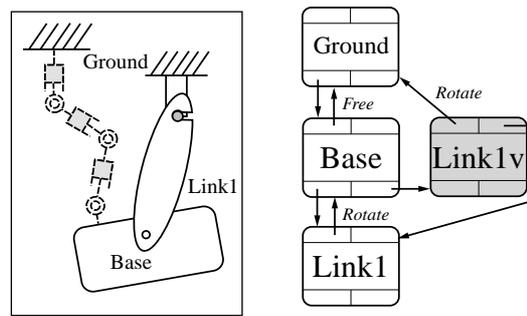
Fig. 8. Closed kinematic chain with free joint
