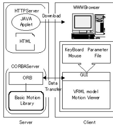
Fig. 14. Configuration of the programming system for the locomotion
