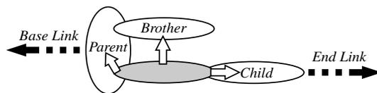
Fig. 1. Three pointers to describe open kinematic chains
