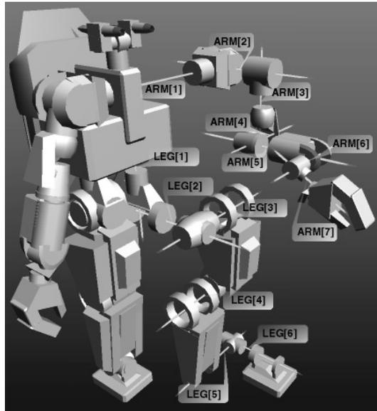
Fig. 18. Configuration of the joints of a humanoid robot
