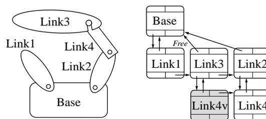
Fig. 9. Link structure and its description after cutting
