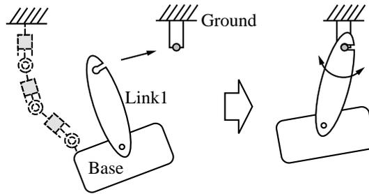
Fig. 6. Open chain generated by link connection
