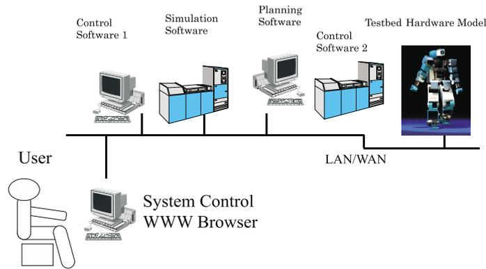
**Fig. 20.** Configuration of V-HRP
