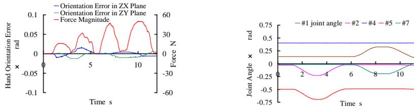
**Fig.14.** Measured Force and Hand Orientation Errors, Joint Angle Changes under Hand Orientation Constraint. This shows the hand orientation errors are slight in spite of large angle change of each joint
