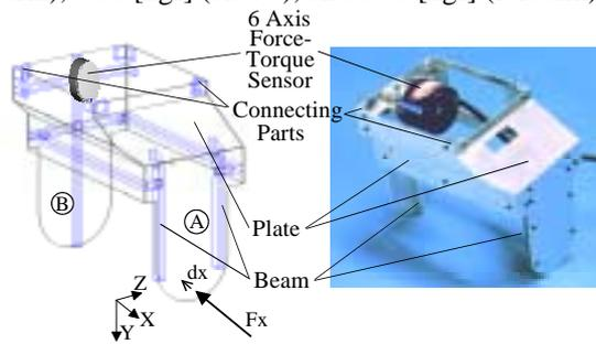
**Fig.4** (i.e.) The Designed and Developed Forearm Surface Cover Module. As a material of the surface cover, 1[mm] light and highly stiff A5052 plate is used. Four plates of A5052 are constructed with L-type connecting parts at the four corners. The surface cover becomes box-typed and each plate is stiffly strengthened with a few beams of which material is YH75
