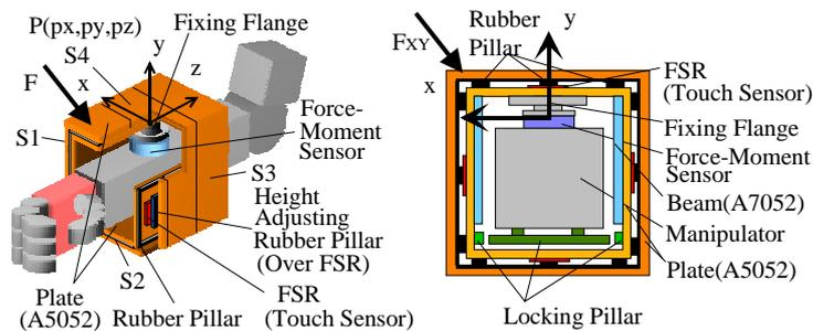
**Fig.3.** Design of Surface Cover. This shows since the box-typed cover is connected with a robot body at a single position for concentrating external force applied onto the cover surfaces to the force/torque sensor. In addition, FSR sensors on the surfaces accurately detect touch information concerning the existence of environments including human
