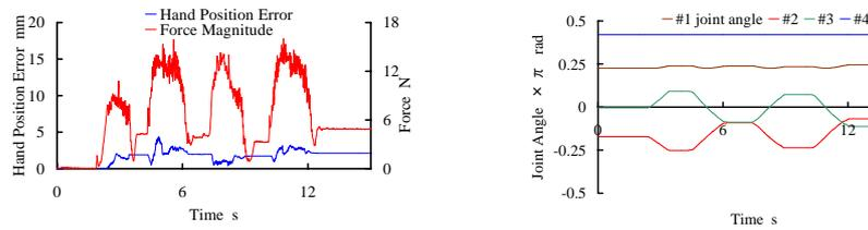
**Fig.15.** Measured Force and Grip Position Errors, Joint Angle Changes under Grip Position Constraint. This shows the grip position error is slight but large amount of force is applied
