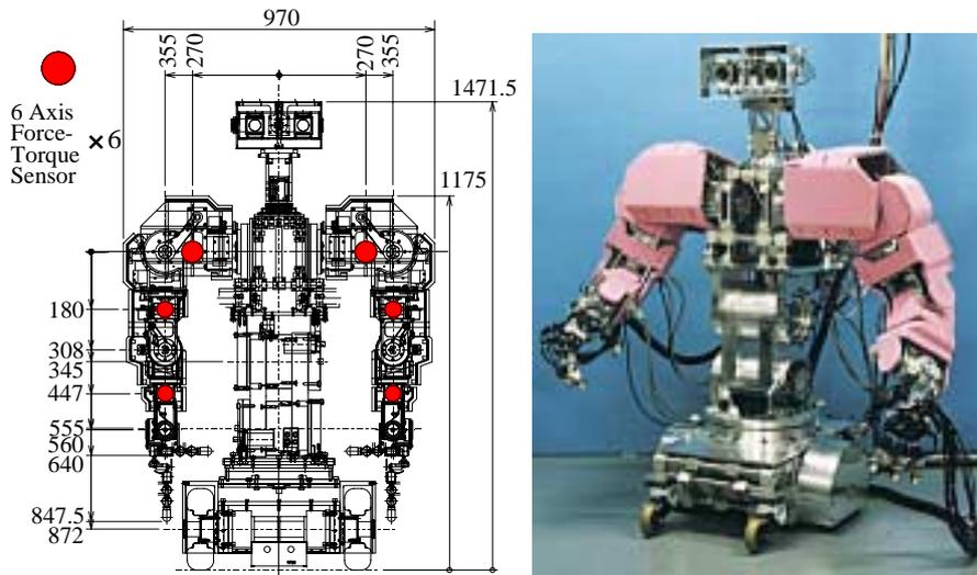
**Fig.5.** Assembly Design and Overview of WENDY with Humanoid Dual Arm Surface Covers
