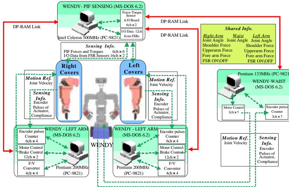
**Fig.7.** PIF Adapting System and Flow of Several Information. The total system is integrated by a host computer and all the processes are conducted at a rate of 1[ms]
